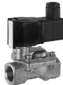
GEMÜ 8258 Servo assisted solenoid valve with pressure differential Brass or stainless steel DN 8 - 15 (0.1 - 16 bar)
