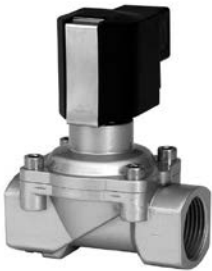
GEMÜ 8253 Servo assisted solenoid valve with a positive lift diaphragm without pressure differential Brass or stainless steel DN 10 - 25 (0 - 16 bar)
